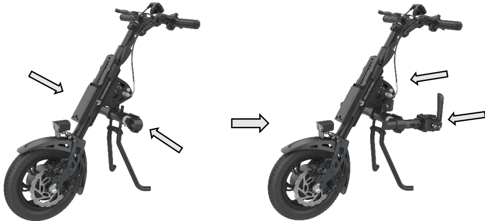
Figure 15. Assembling the Manual Clamp Assembly
